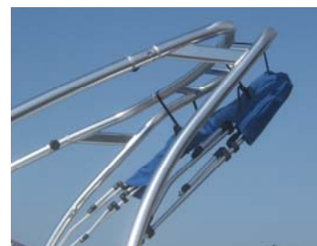
Tower Bimini. Stored Position
